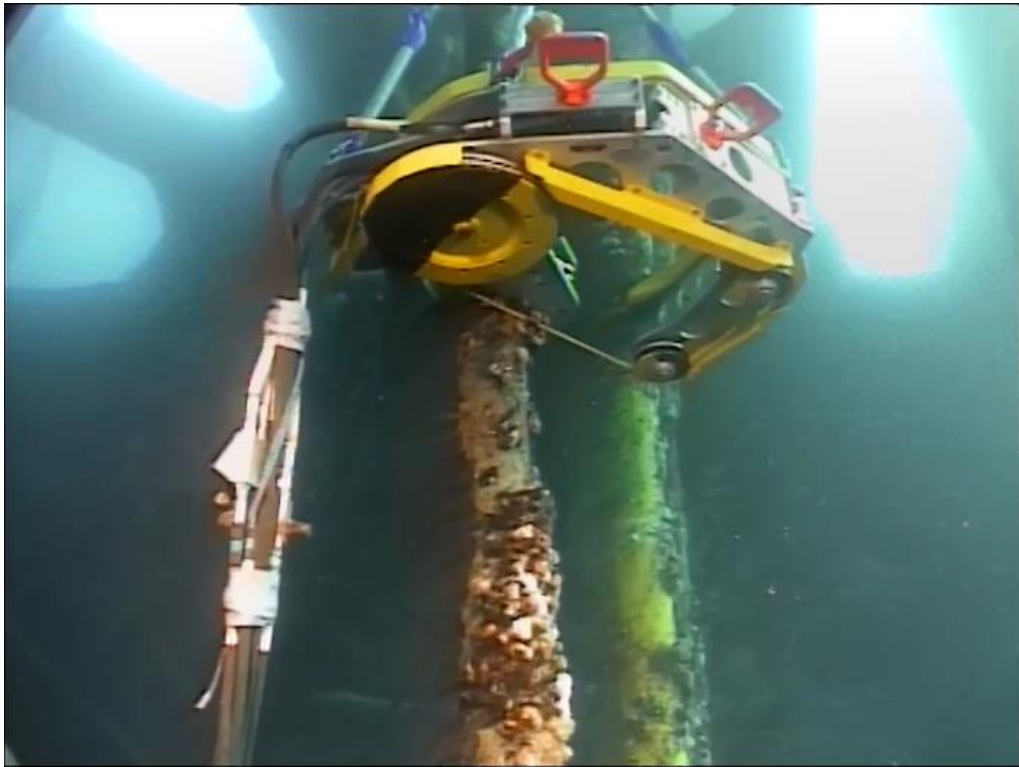
Figure 9.3.1: DWCM in position on riser PL2574
