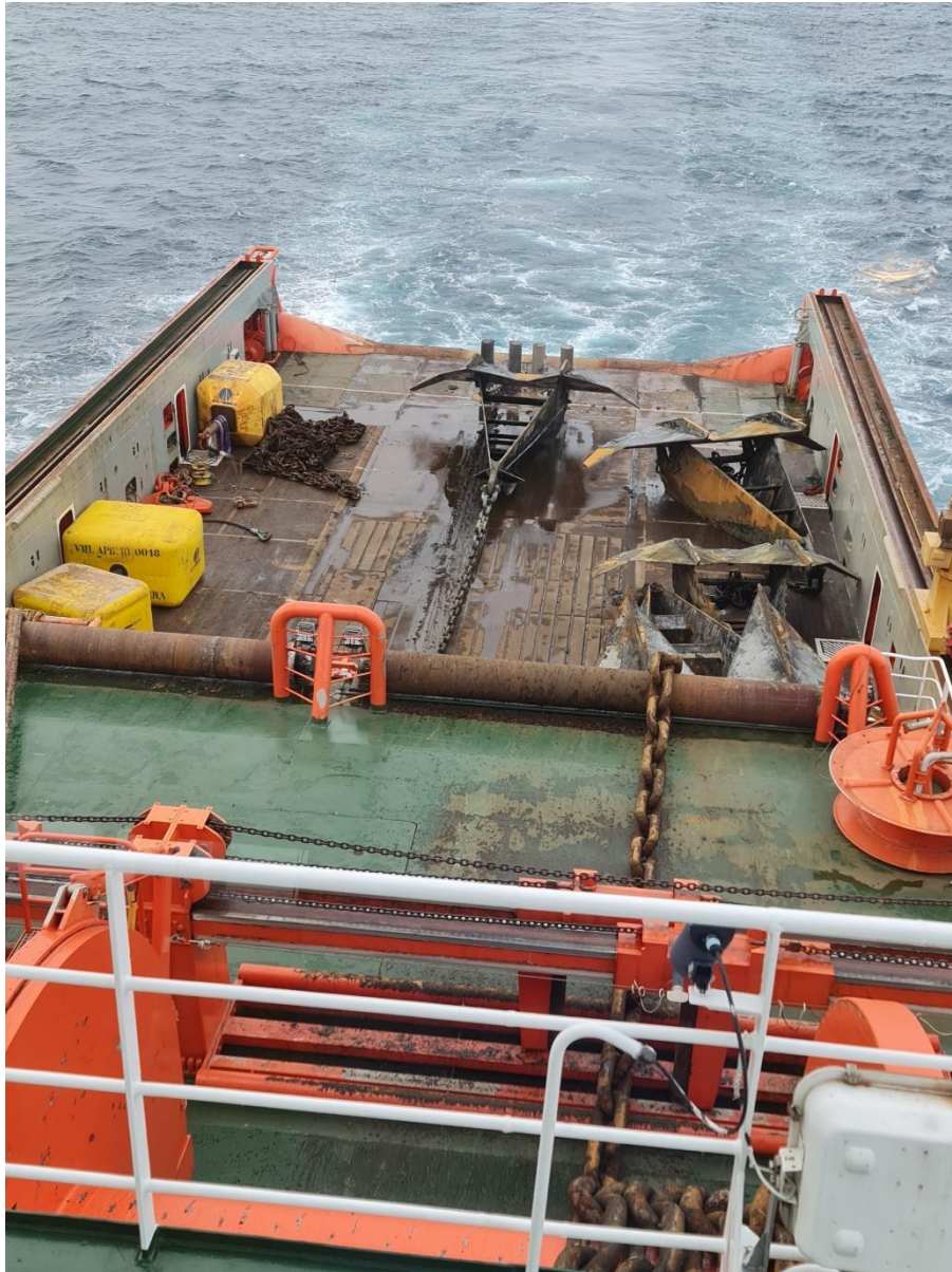
Figure 9.2.1: Northern Producer anchor & chain recovery
