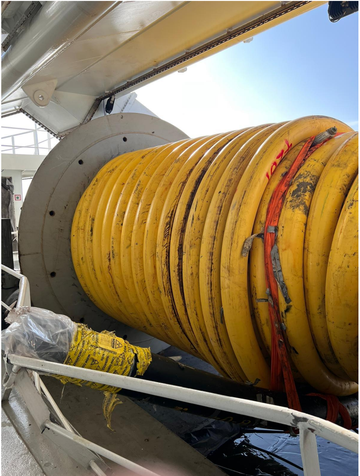
Figure 9.4.1: Umbilical riser on AHV drum
