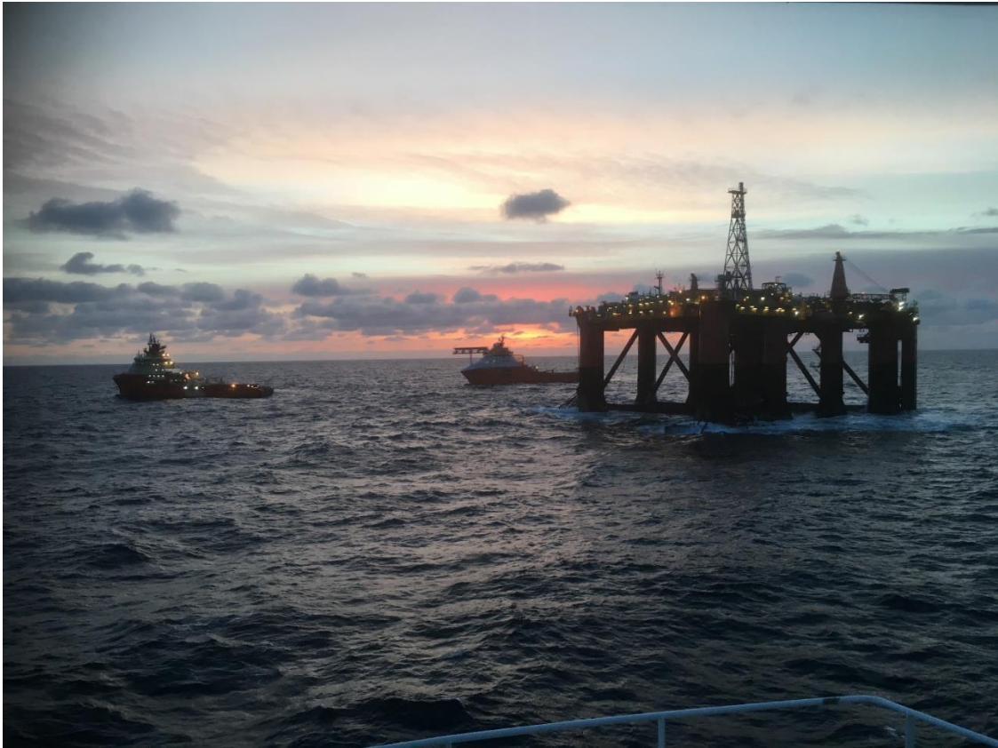
Figure 9.1.1: NP FPF under tow using Anchor Handler Vessels ('AHV')
