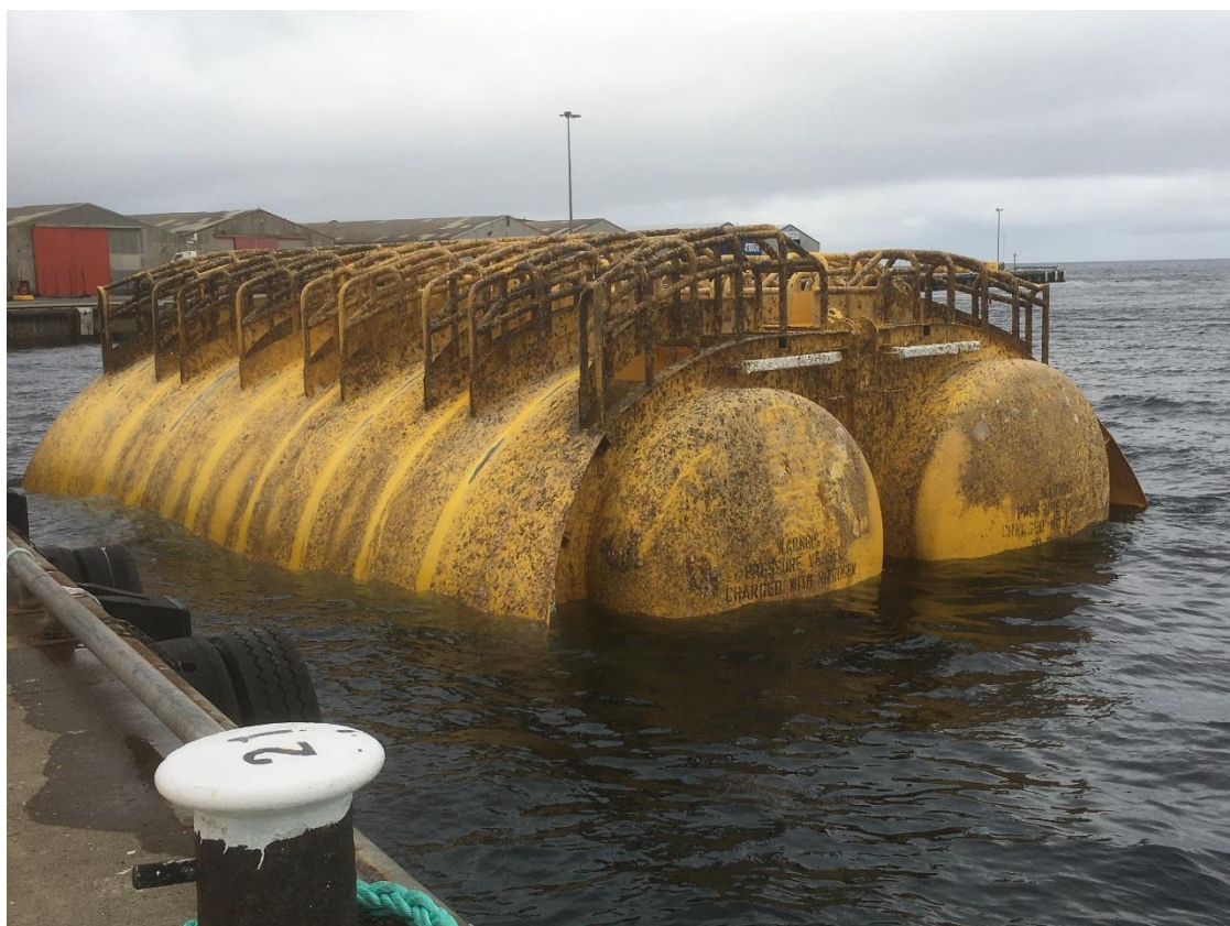
Figure 9.5.3: Mid-Water Arch alongside quayside
