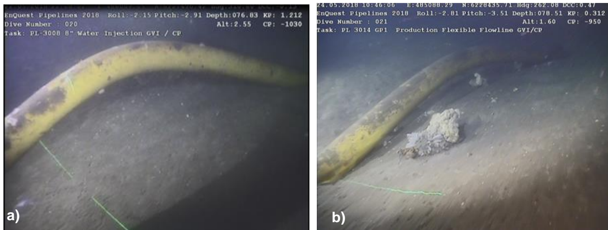
Figure 2.1.2: Image of freespan at KP1.212 (PL3008) and KP0.312 (PL3014)
